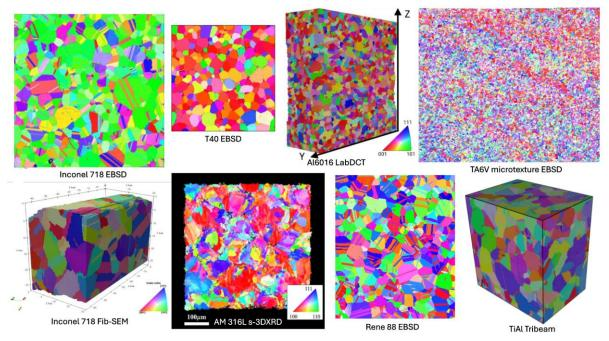
Above figure: examples of various metallic polycrystalline microstructures, including steel, aluminium, titanium and nickel based alloys; these microstructure were characterized by electron of X-ray diffraction, in 2D (surface) or 3D (tomography). All images are depicted using inverse pole figure coloring related to the crystal orientation.
